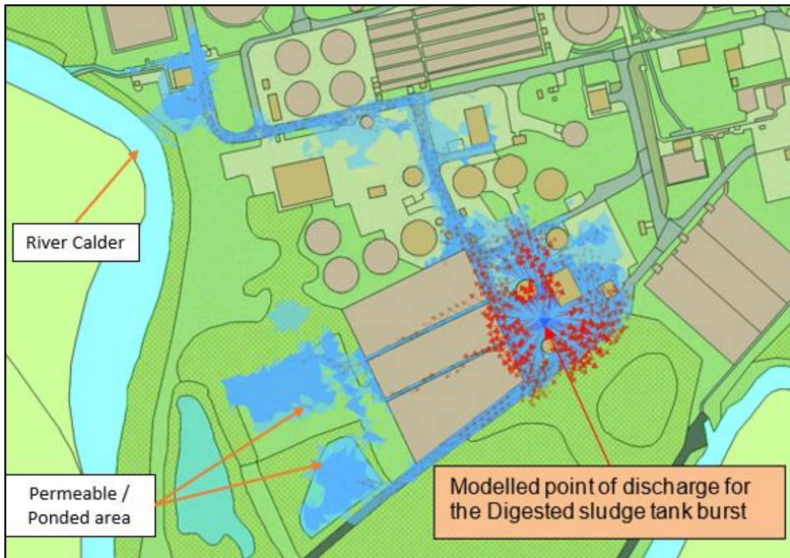
Figure 11 Burnley STC Predicted Flow Paths following Digested Sludge Tank Burst
