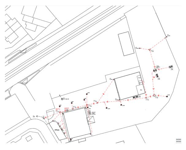
The drain plan shows the combined surface water & foul water drainage and interceptor system and direction of flow for the site.
