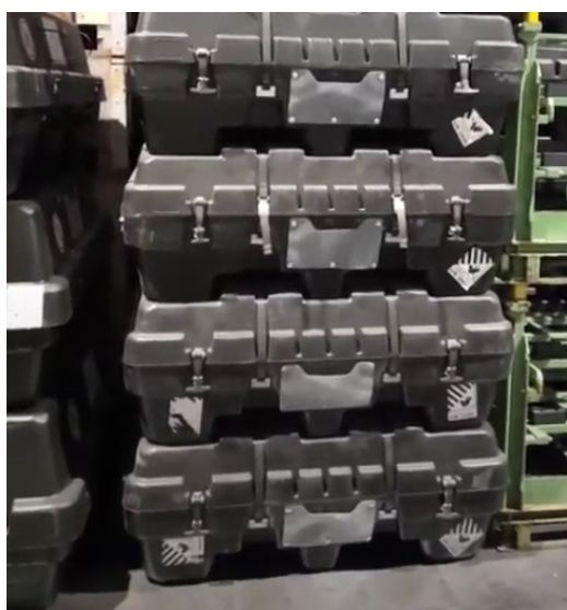
Figure 2. Example of weatherproof battery containers
