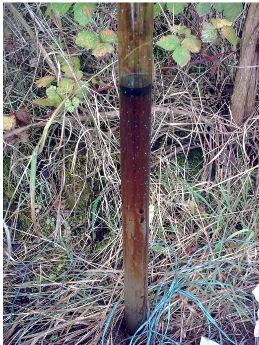
Photograph 10: Free phase oil product in bailer from BH221a (August)
