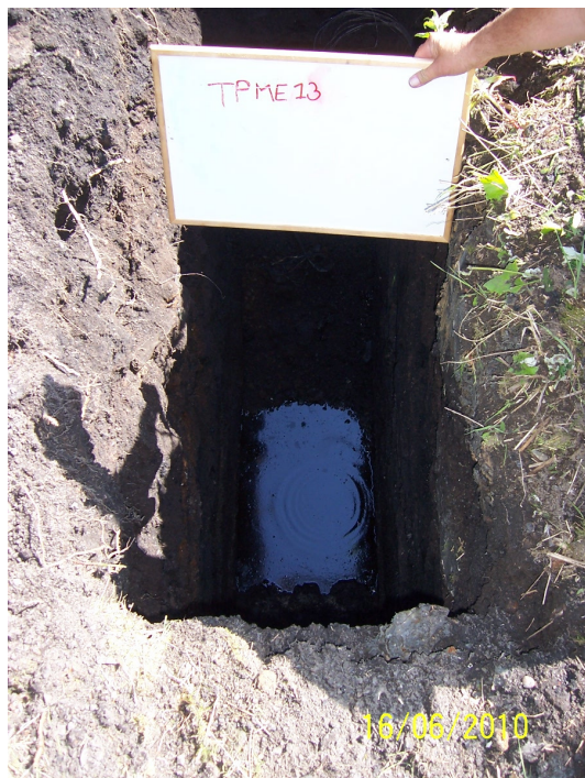
Photograph 6: Pooling oily liquid at the base of TPME13
