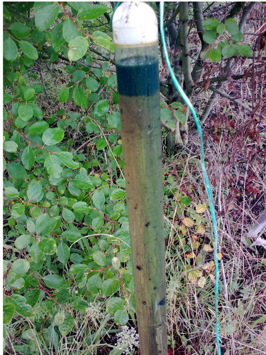
Photograph 9: Free phase oil product in bailer from BH107 (August)
