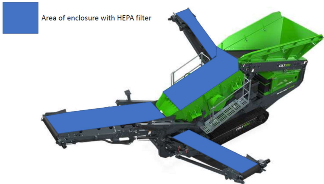
Figure 3. Areas of Covering on Soil Screener
