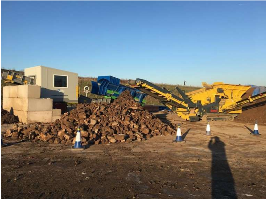
Figure 7. Soil Screening and hand picking of soil (Maw Green)
