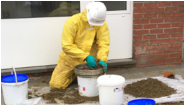
Asbestos sampling activities in Belgium | AECOM
