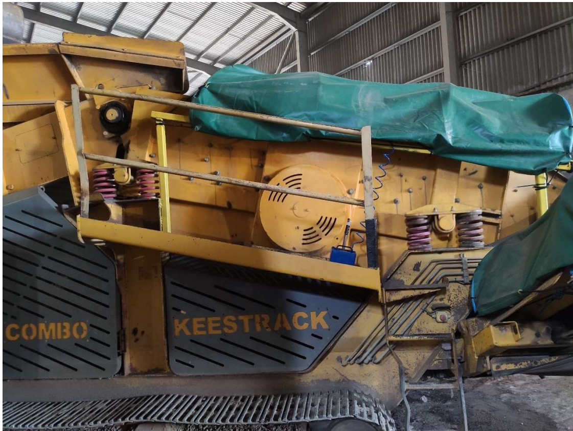
Figure 4. Covers on screener, note the asbestos monitoring pump located under the sheet on the screener deck
