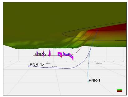
Cross sectional view looking due North across the PNR2 wellbore. The modelled fractures can be seen growing away from the well bore, this represents the complete fracture model not just the average fracture height. The upper limit of the permitted boundary is shown by the contoured horizon, blue representing deep moving into yellow at shallower depths. A grid is provided for scale, each box has a side length of 800m.
