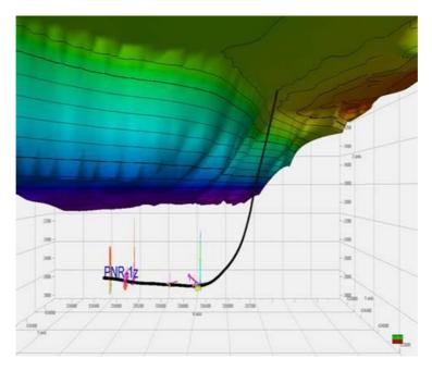
Cross sectional view looking due North across the PNR1z wellbore. The modelled fractures can be seen growing away from the well bore, this represents the complete fracture model not just the average fracture height. The upper limit of the permitted boundary is shown by the contoured horizon, blue representing deep moving into yellow at shallower depths. A grid is provided for scale, each box has a side length of 200m.
