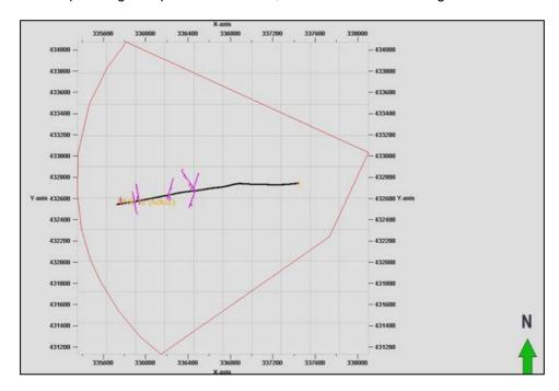
Map view of the permitted boundary, PNR1z wellbore shown in black and the hydraulic fracture models shown in purple.
