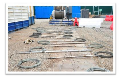
Seismic waves are recorded using seismometers or geophones. The image (left) shows the array of borehole geophones before they were positioned in the second well at the site. They measure the fracturing of rock. This equipment can detect the very small levels of micro seismic activity underground. Additionally there are surface monitoring seismic sensors.
