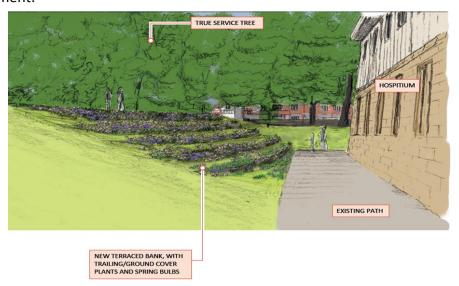
As the works move back towards Marygate this will involve the creation of a larger area of terracing behind the Hospitium. This terracing is made up of pre-seeded greenfix sandbags containing a native grass/seed mix and will be further enhanced by the Landscape planting scheme due to start next spring.
