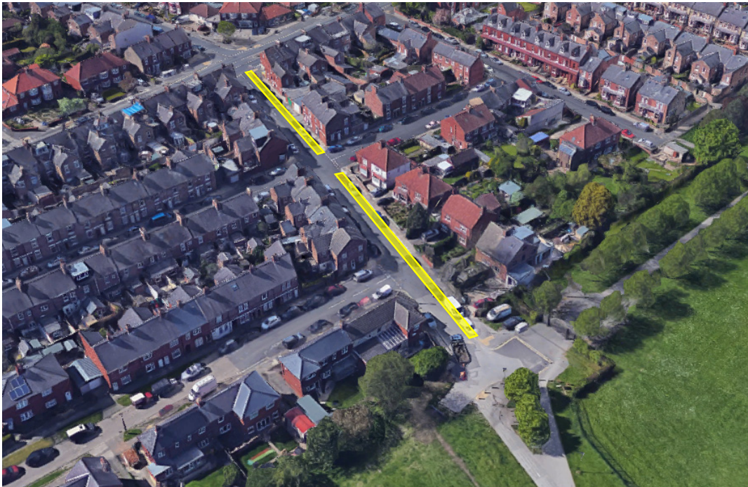
Figure 10 - Plan view showing proposed parking bay suspensions on northern side of Butcher Terrace
