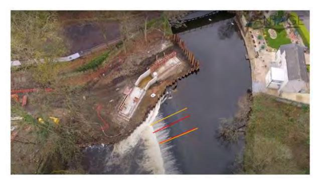
Figure 62 Plan view of breach progression (red = pre 06-02-2021, yellow = post 06-02-2021)
