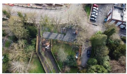
Cadent Gas works are ongoing to divert the gas main around the wall foundations, adjacent to the bridge.
