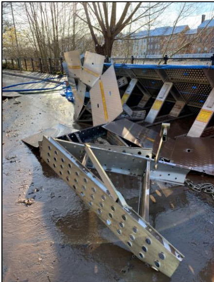
Figures 18 and 19: Section of barrier where the breach occurred twisted back, a weld was observed to be broken.
