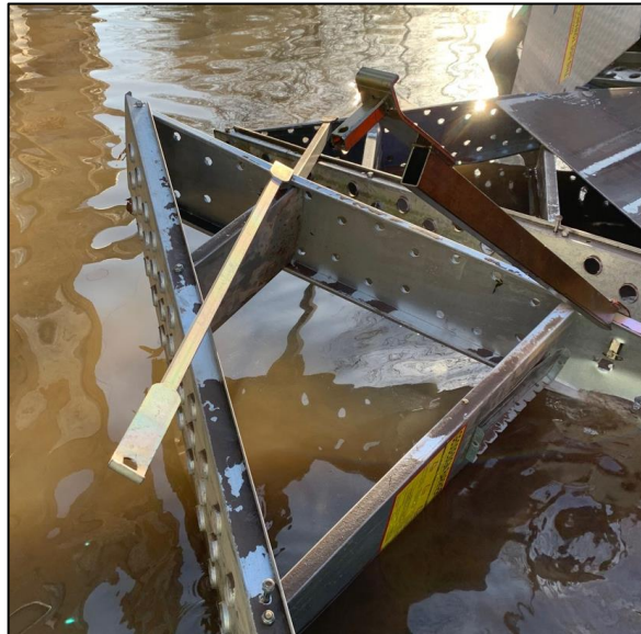
Figures 18 and 19: Section of barrier where the breach occurred twisted back, a weld was observed to be broken.
