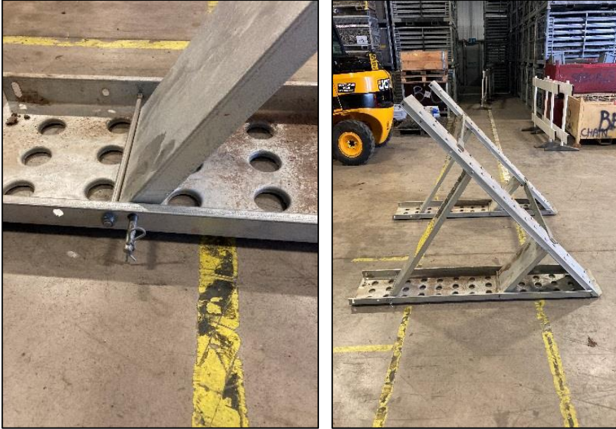
Figures 7 and 8: Barrier feet with protruding 'collars' which make contact with the surface below.
