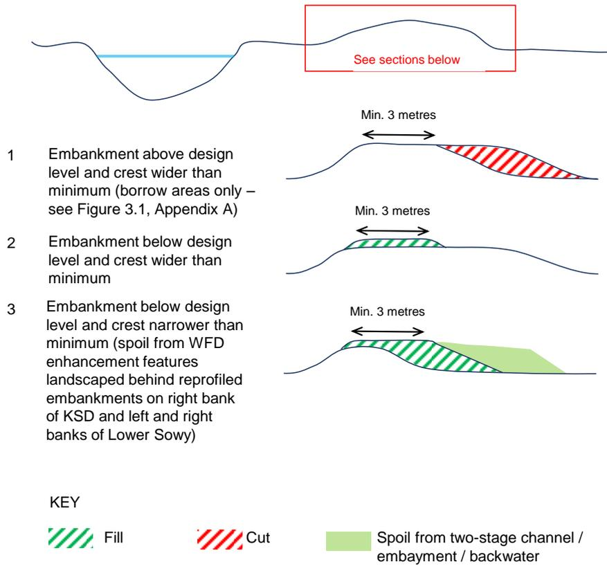
Figure 2 Schematic illustration of bank re-profiling process
