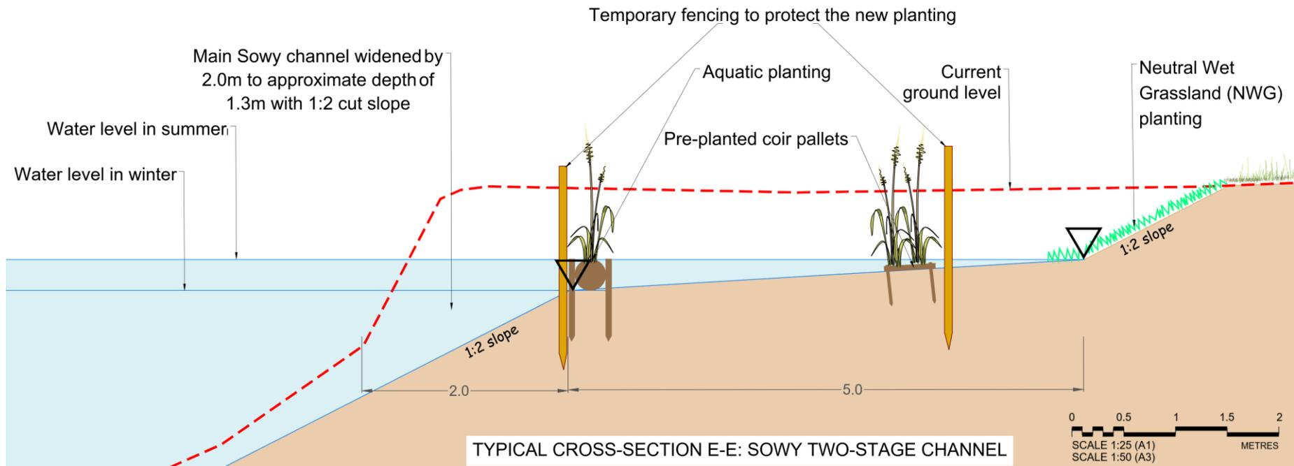
Figure 3 Example cross section of a two stage channel which will be created on the eastern side (right bank) of the Sowy
