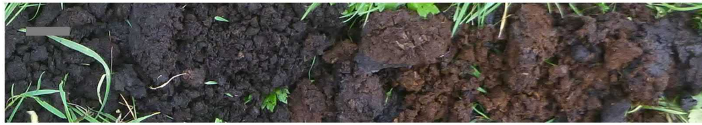
Junction of black oxidised peat with reduced peat at 0.8m bgl BH20.
