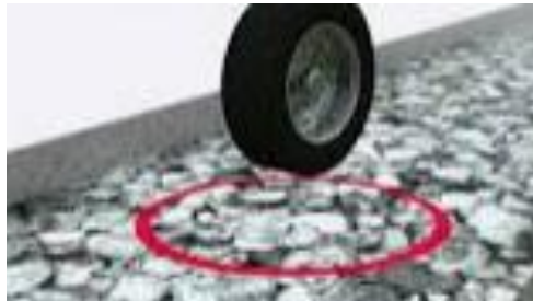
Figure 8: Wheel load distribution modelled as circular footing
