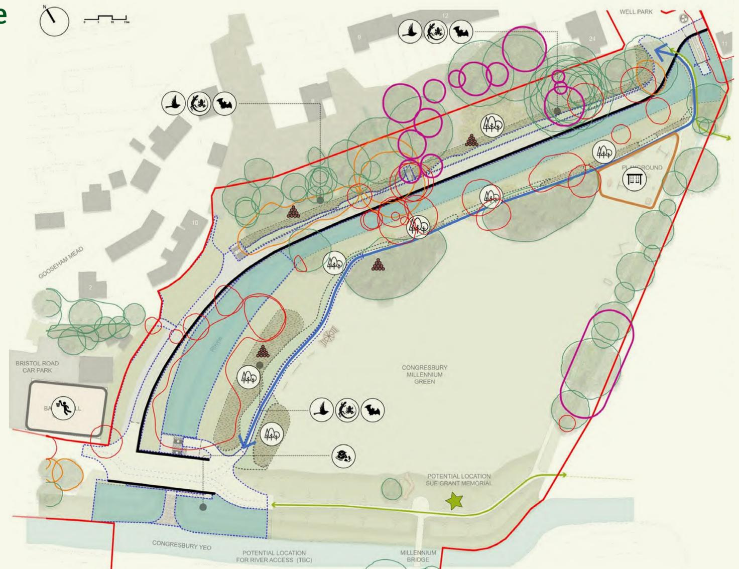
The rhyne re-alignment has been designed to provide aquatic ecological benefit through the creation of a two-stage channel, which will encourage aquatic wetland species to grow at the channel margins.
