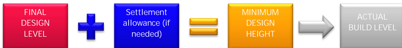
Figure 3.2: Application of settlement allowance
