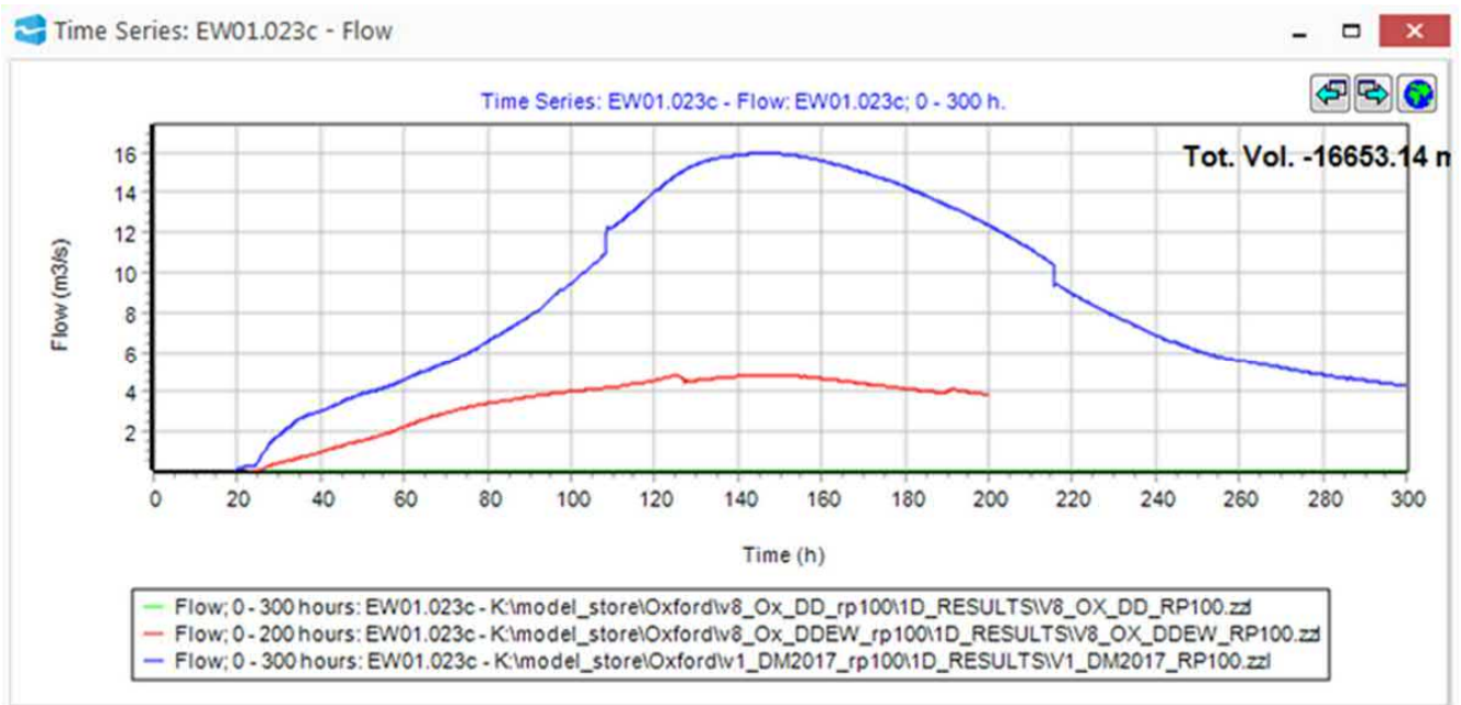
Figure K.2: 1% AEP flows through the railway culvert upstream of Eastwyke ditch control structure
