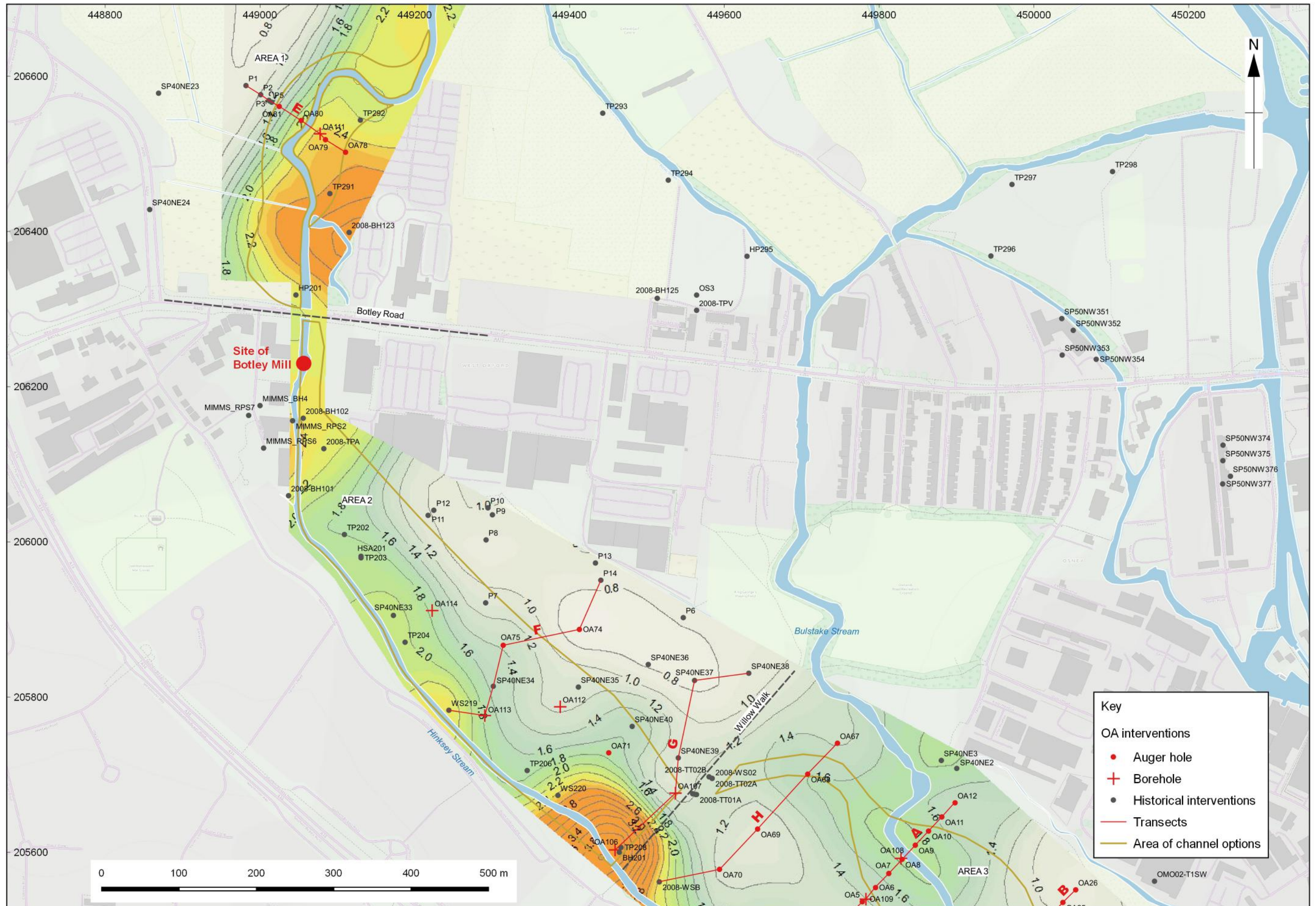
Figure 8: Modelled thickness (m) of deposits overlying gravel surface (based on borehole and auger data), Areas 1 and 2
