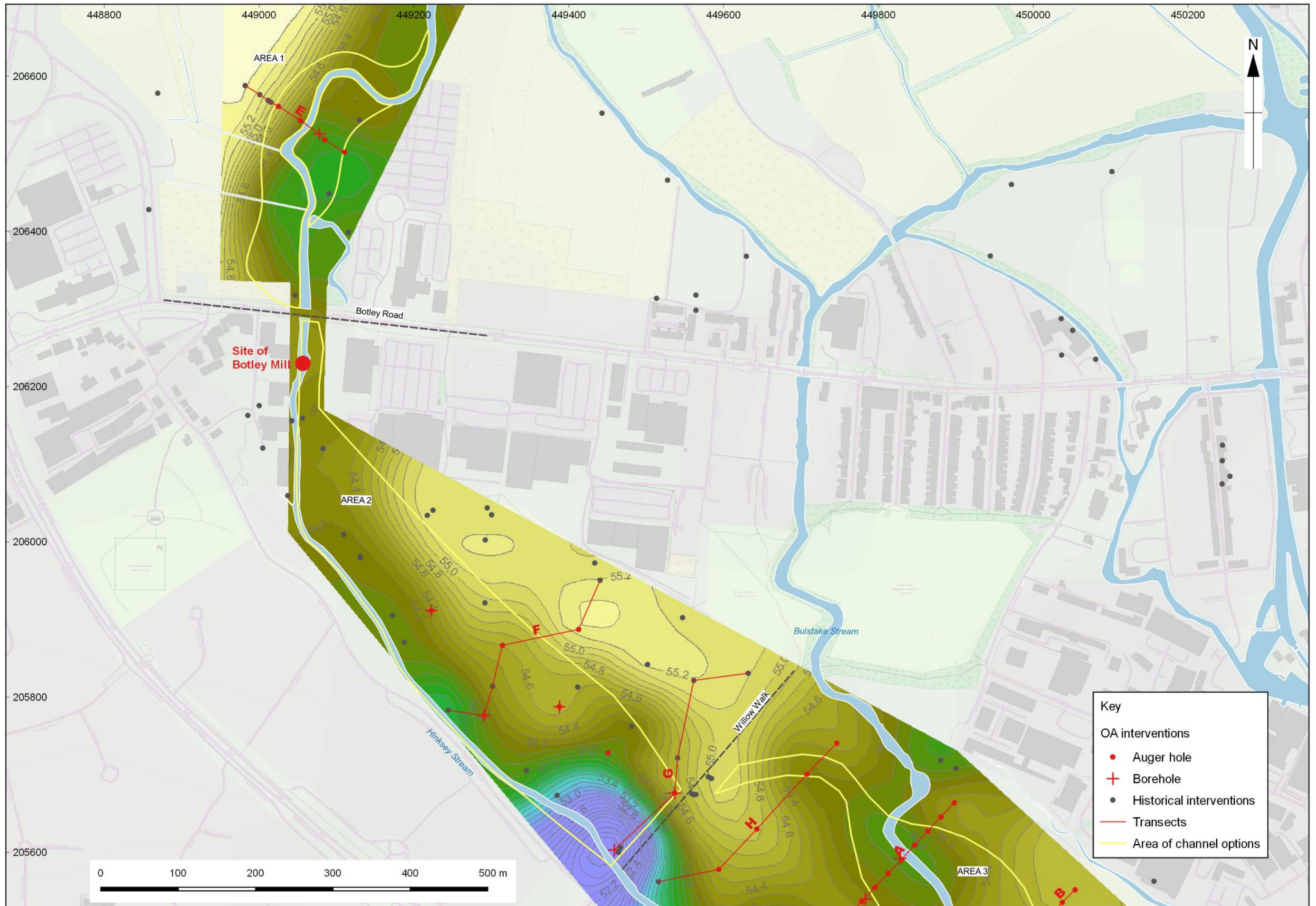
Figure 6: : Model of gravel surface (m OD) based on borehole and auger data, Areas 1 and 2
