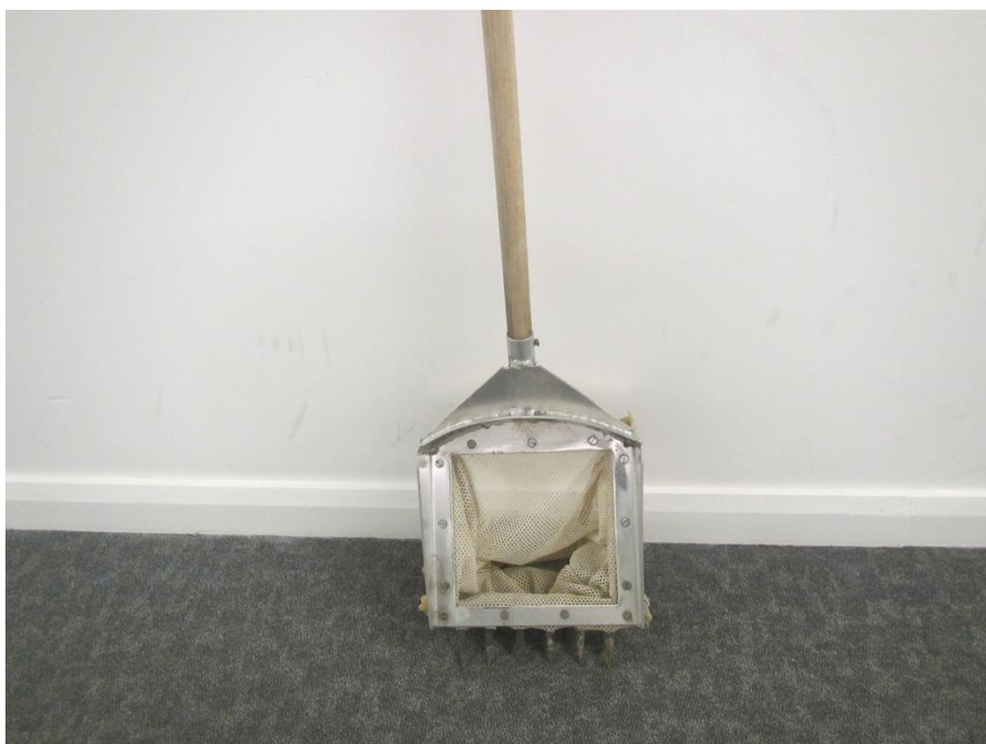
Plate B16: Modified pond net used for Unionidae surveys
