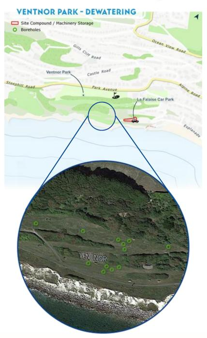
Above Ventnor's Western Cliff we will install subsurface monitoring equipment and drill an abstraction borehole, before undertaking a pump test to inform us about water quality, extractable quantities, and groundwater behaviour. It is important that this work starts as early as September so that we can collect data over winter when groundwater levels are highest.
