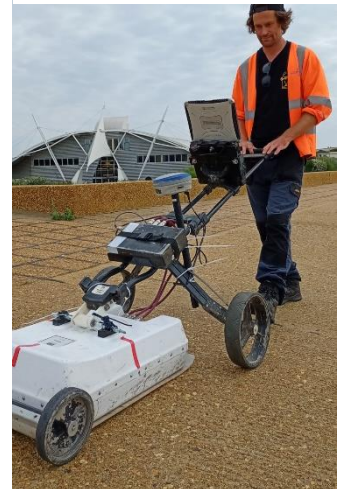
Figure 2 - GPR equipment used in Sandown Bay. Image submitted by a member of the public.
