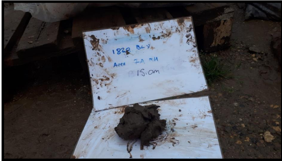
Area 7A BH Sample at 15.0m
