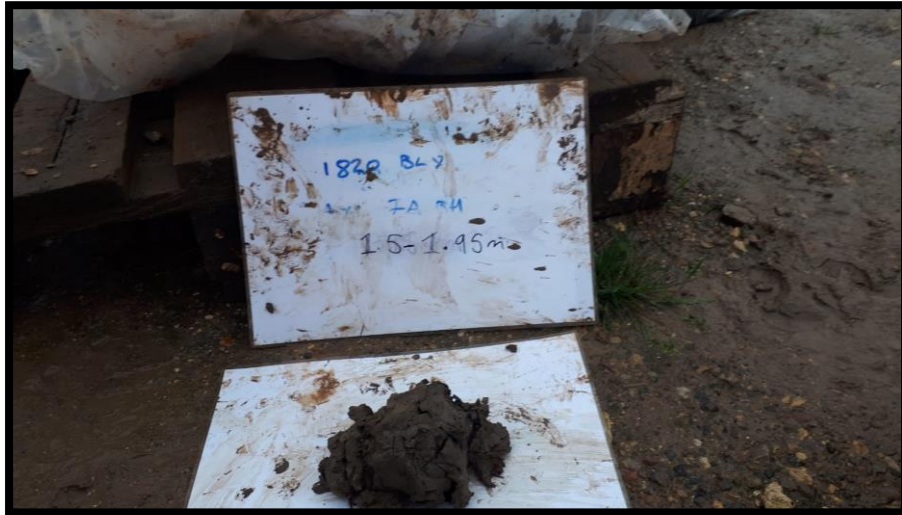
Area 7A BH Sample at 1.5 - 1.95m
