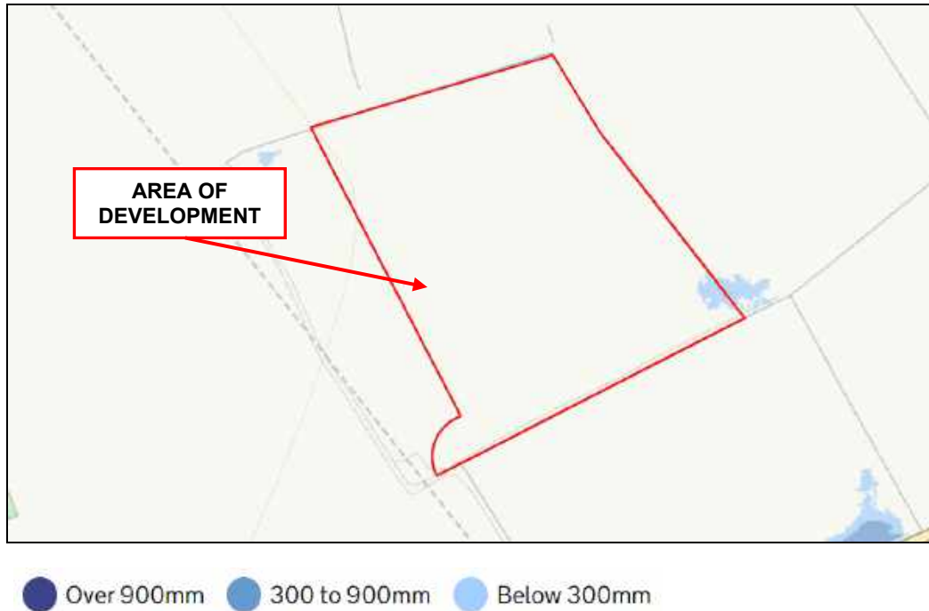
Figure 6: Environment Agency map dated October 2021 showing the likely depth of flooding from surface water – low risk
