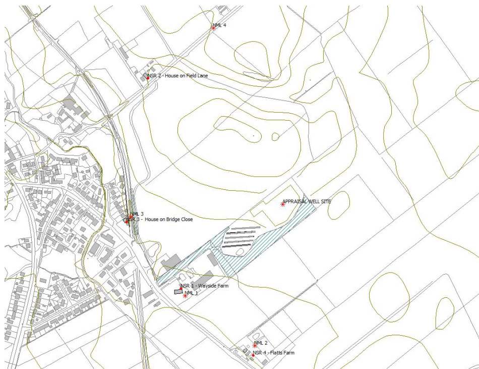
Figure 3: Noise sensitive receptors (NSR 1-4) and noise monitoring locations (NML 1-2 unattended; NML 3-4 attended). Weather station located at NML 2
