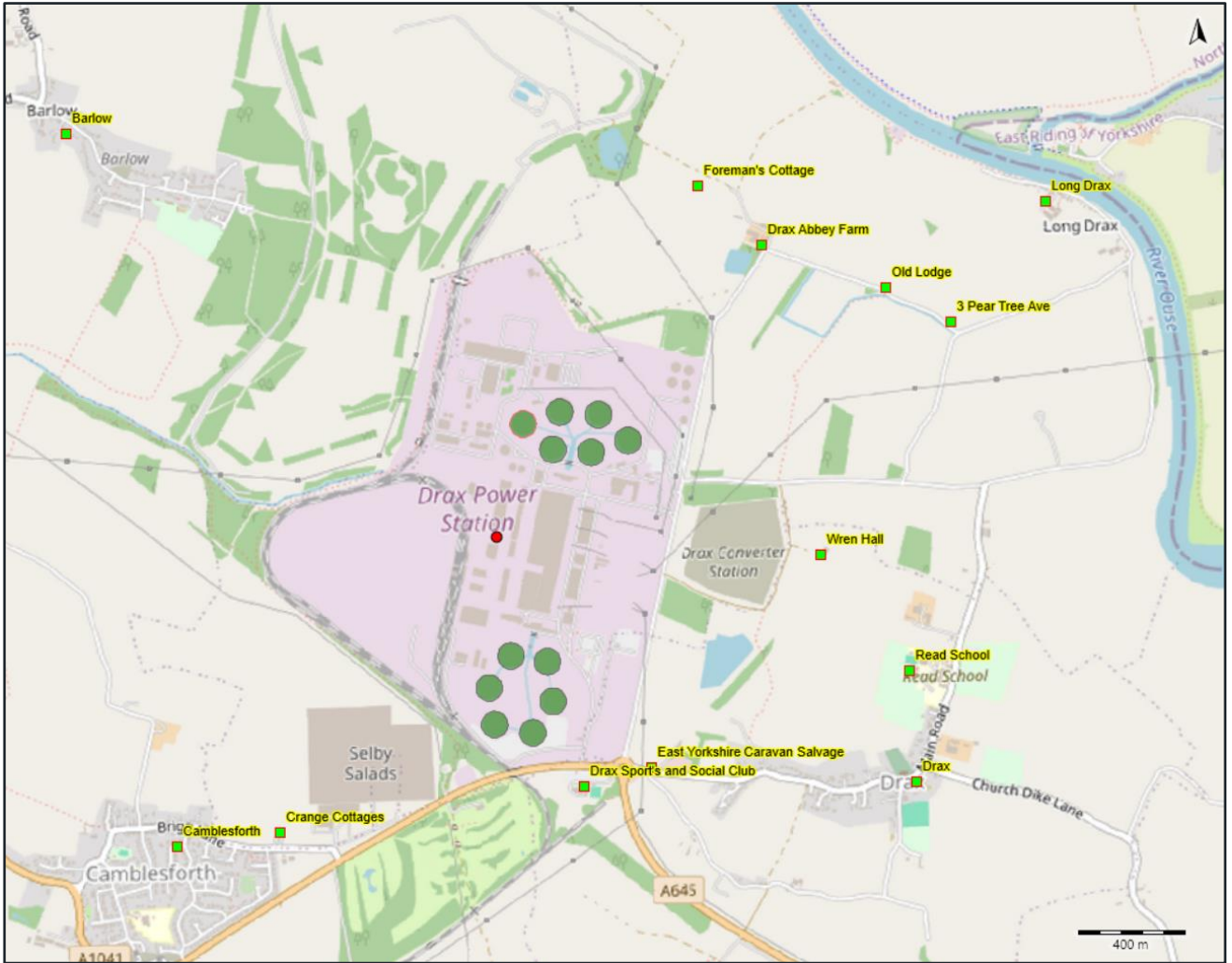
Figure A-3 - Illustrative receptors for human health effects in the vicinity of Drax power station (green filled squares). The Drax main stack is shown as a red filled circle. Buildings included in the modelling are shown as dark green filled circles.
