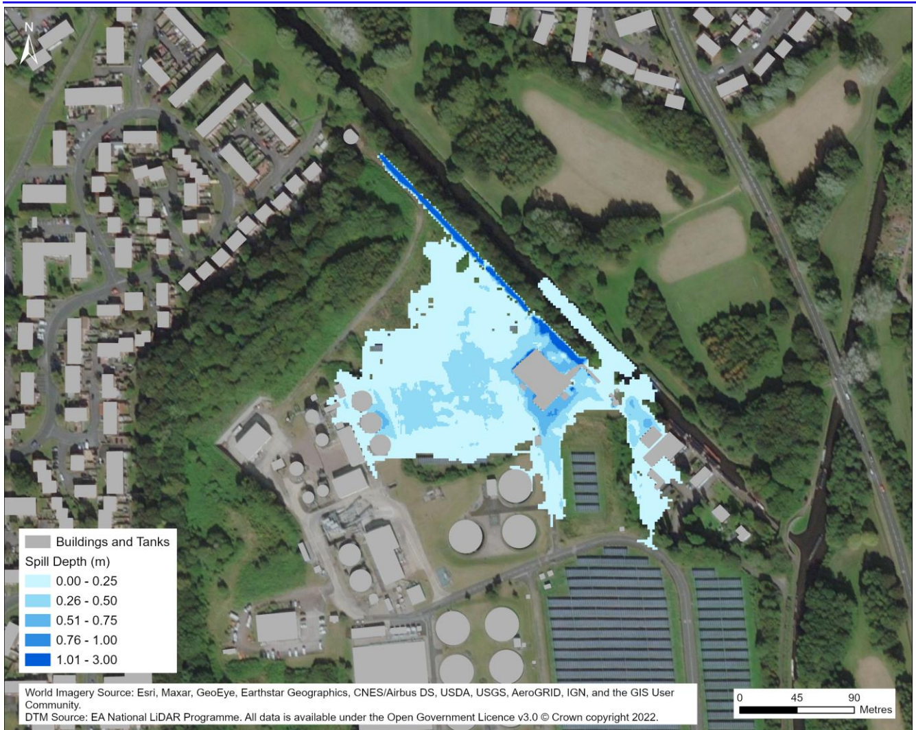
Figure 2.3 Uncontrolled spill of Barnhurst Sewage Treatment Works (Depth profile)
