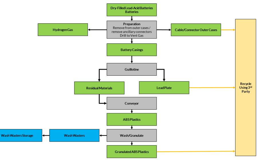
Process flow for the Mixed Battery treatment procedure undertaken at Fenix. Detailed information on the treatment process can be found in section 2.1 of the *Waste Treatment Procedure* (FEN-OP03).
