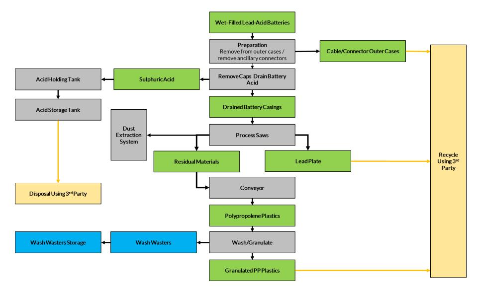
Process flow for the Dry-Filled Lead-Acid Battery treatment procedure undertaken at Fenix. Detailed information on the treatment process can be found in section 2.4 of the *Waste Treatment Procedure* (FEN-OP03).
