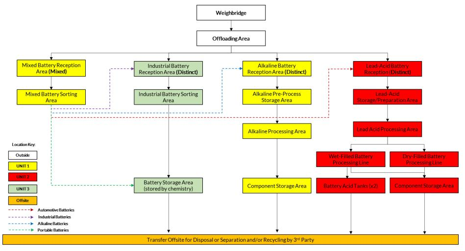
Process flow for the Alkaline Battery treatment procedure undertaken at Fenix. Detailed information on the treatment process can be found in section 2.2 of the *Waste Treatment Procedure* (FEN-OP03).
