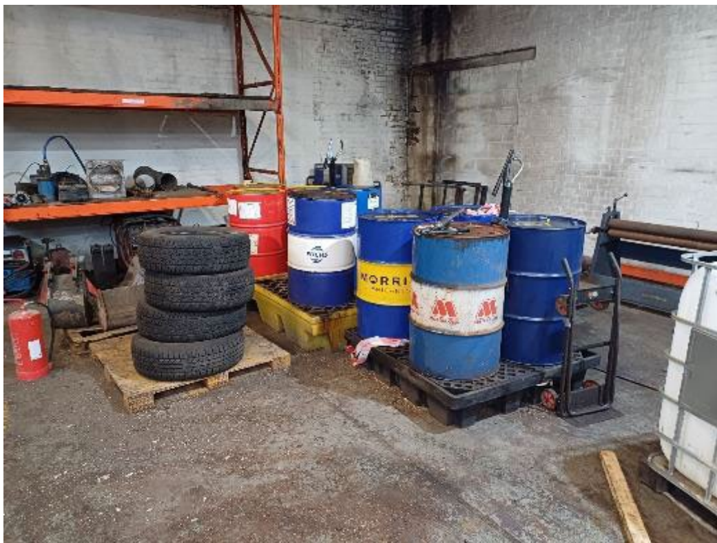
Photograph 9: Oil drums stored on bunded pallets in the Maintenance Room within the internal Additional Area.
