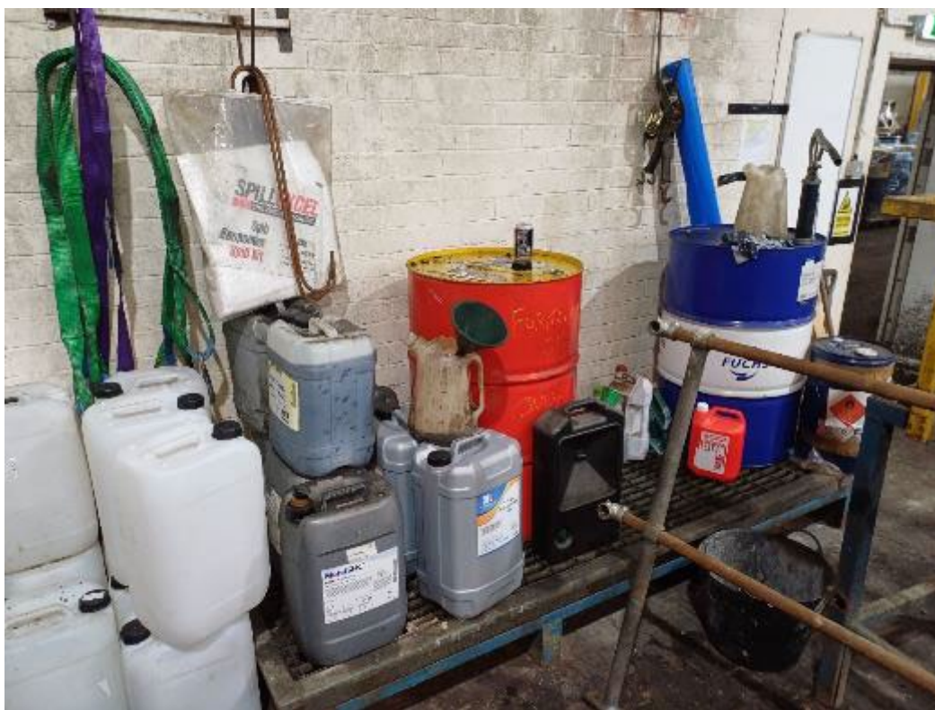
Photograph 10: Oil drums/containers stored on bunded pallets in the Maintenance Room within the internal Additional Area. Spill kit noted also.
