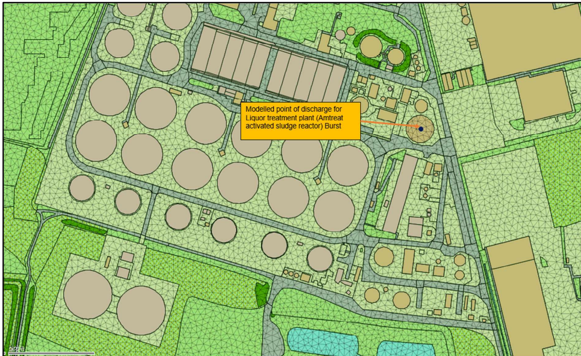
Figure 12 Leigh STC Modelled Point of Discharge for Liquor Treatment Plant (Amtreat activated sludge reactor) Burst
