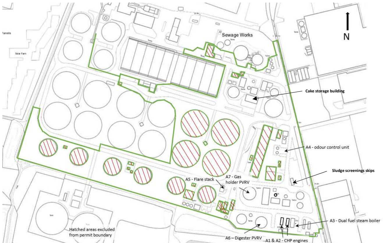
Figure 3.1.1 Map of site showing the location of the OCU, screening skips and cake storage building
