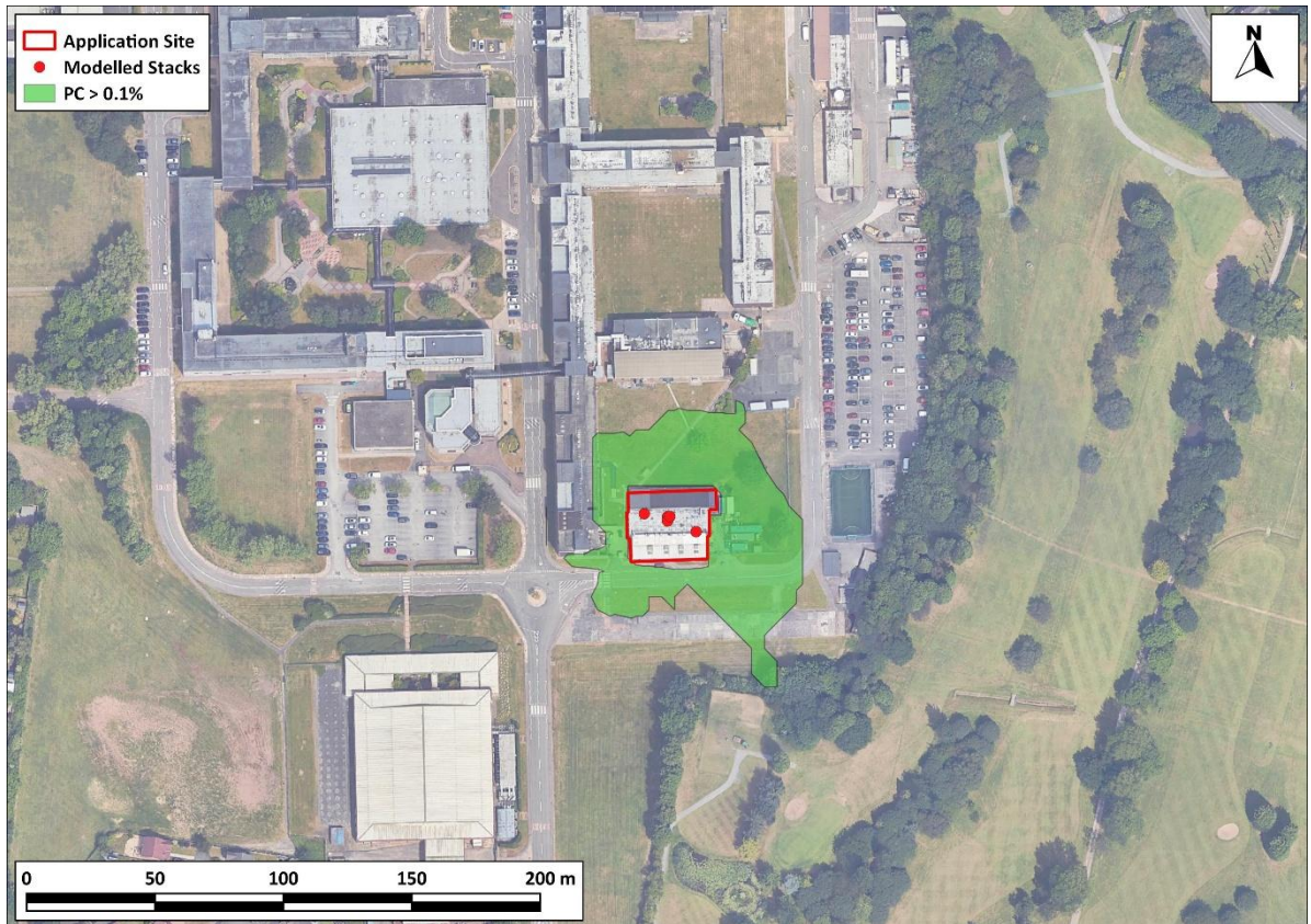
Figure A2-3: Contour Plot of the 8-hour Rolling Mean CO PCs
