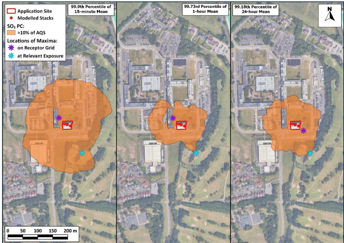
Figure 8-7: Contour Plots of SO 2 PCs and Locations of Maxima on Entire Grid and at a Relevant Receptor for Each Averaging Period (15-minute, 1-hour and 24-hour)
