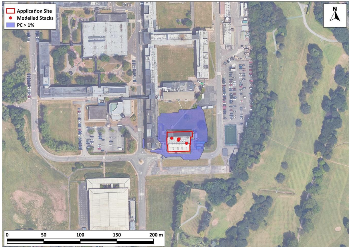
Figure A2-9: Contour Plot of the 1-hour Mean HF PCs
