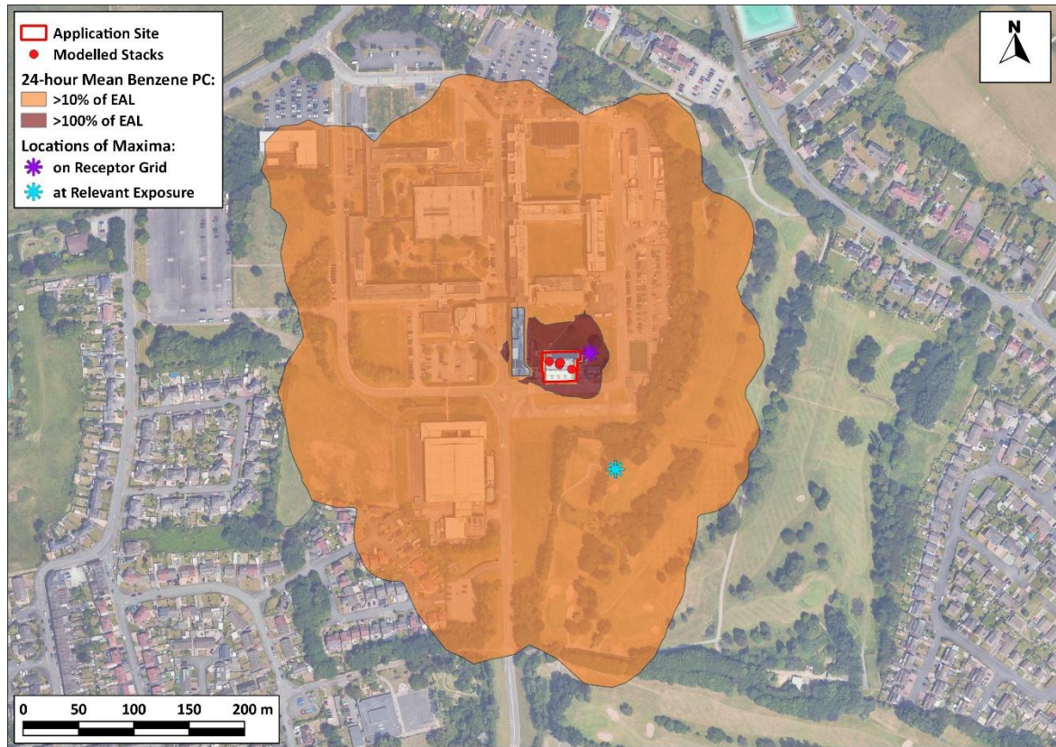
Figure 8-6: Contour Plot of 100 th Percentile of 24-hour Mean Benzene PCs and Locations of Maxima on Entire Grid and at a Relevant Receptor
