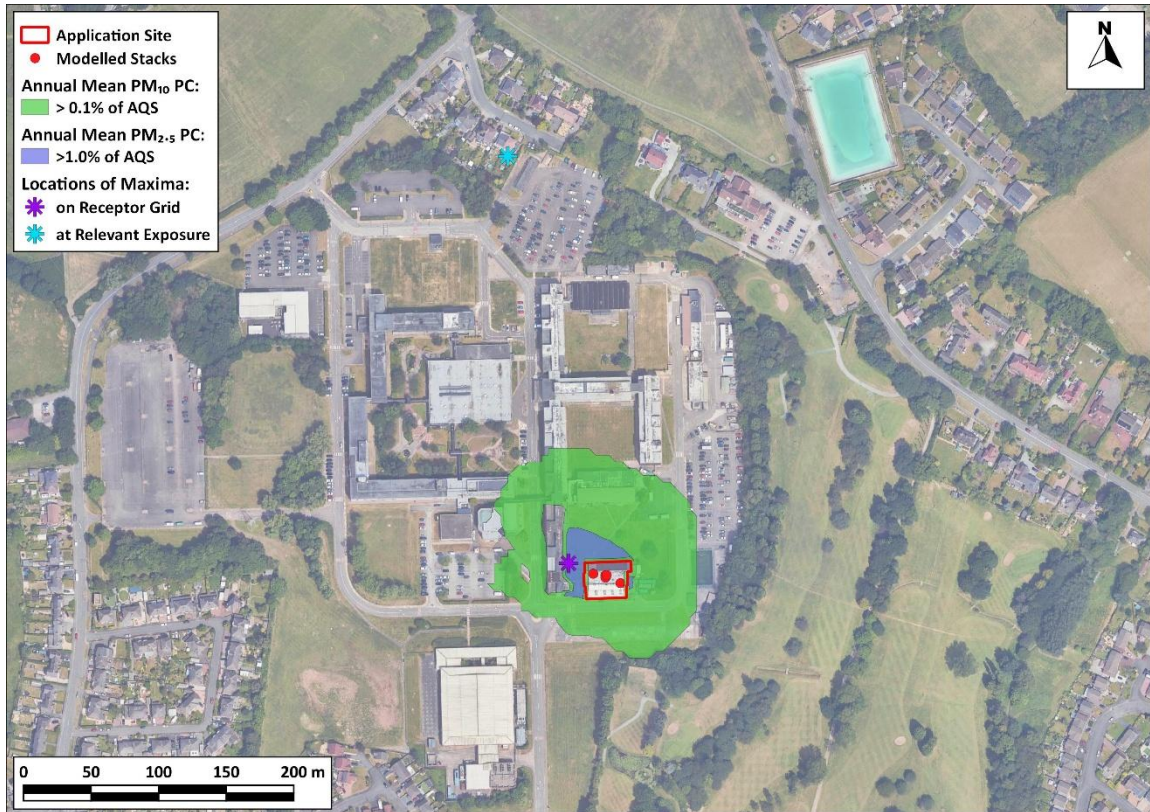
Figure 8-1: Contour Plot of Annual Mean PM_{10} and PM_{2.5} PCs and Locations of Maxima on Entire Grid and at a Relevant Receptor
