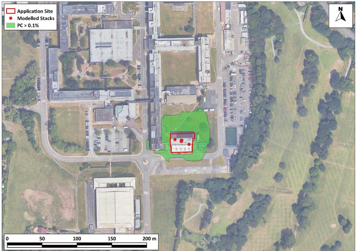
Figure A2-4: Contour Plot of the 1-hour Mean CO PCs
