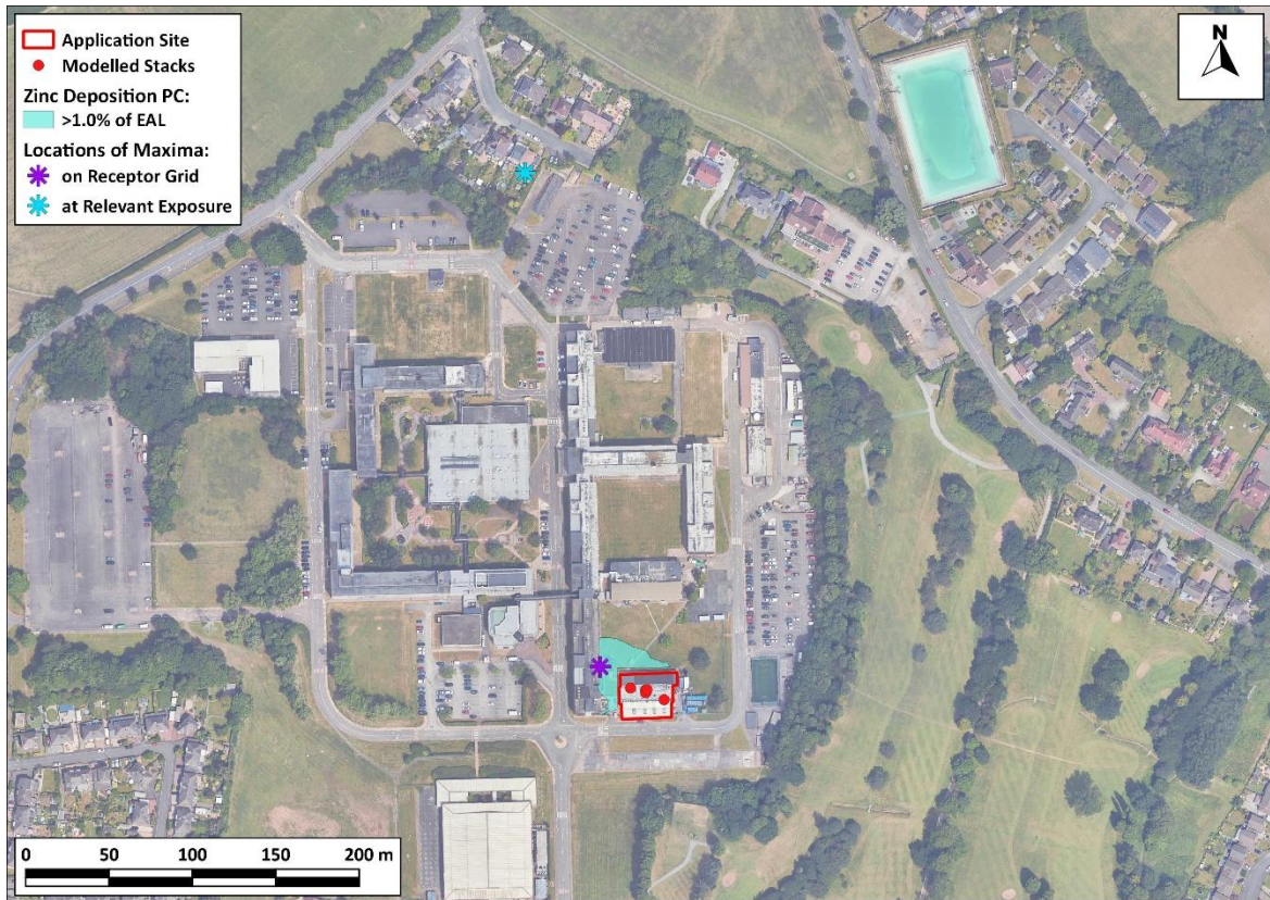
Figure 8-11: Contour Plot of Zinc Deposition PCs and Locations of Maxima on Entire Grid and at a Relevant Receptor
