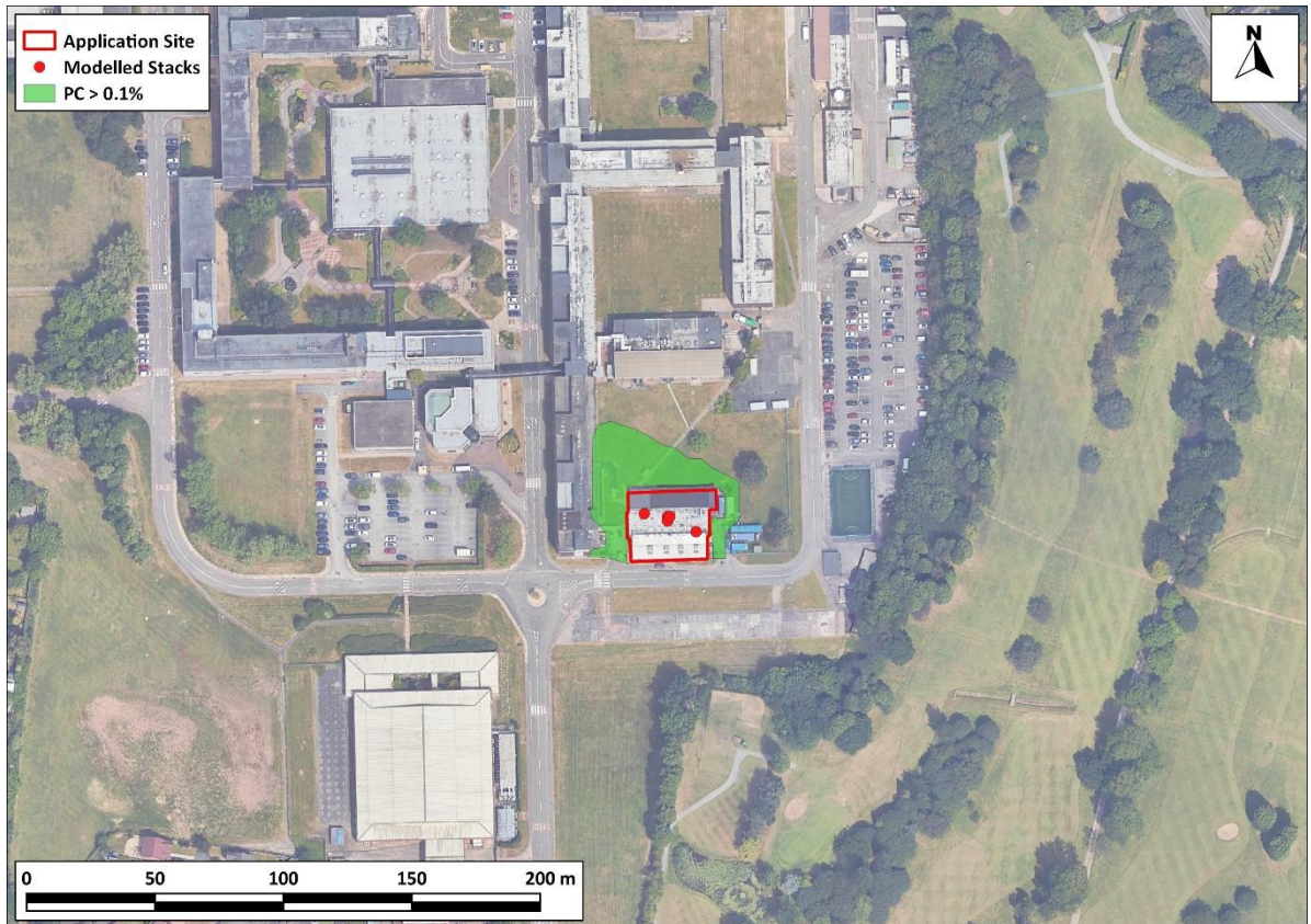
Figure A2-1: Contour Plot of the Annual Mean Methanol PCs
