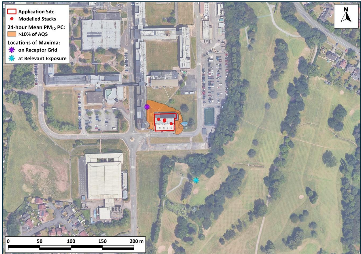
Figure 8-5: Contour Plot of 90.4 th Percentile of 24-hour Mean PM 10 PCs and Locations of Maxima on Entire Grid and at a Relevant Receptor
