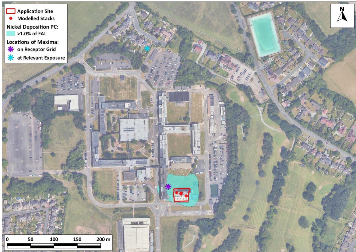
Figure 8-10: Contour Plot of Nickel Deposition PCs and Locations of Maxima on Entire Grid and at a Relevant Receptor
