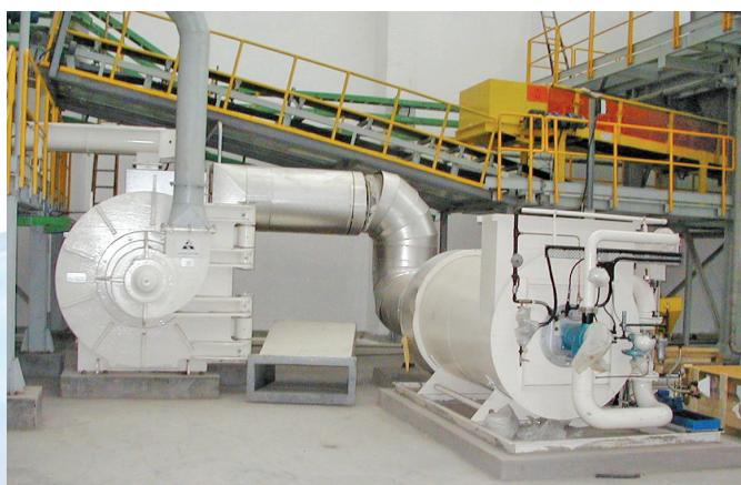
An 18A Dryer-Pulveriser and gas-fired air heater for processing precipitated calcium carbonate (PCC)
