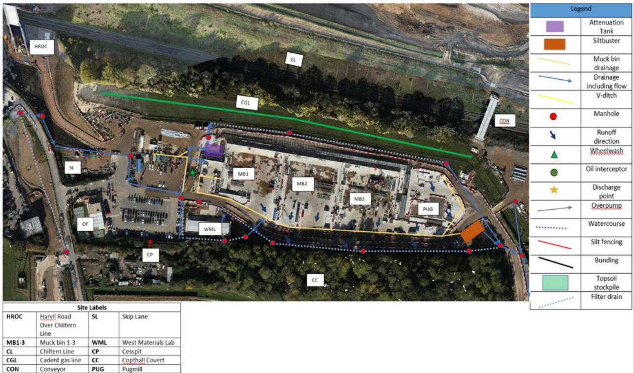
Figure A3.3: Southern Treatment Area and Skip Lane Drainage Diagram with Map Diagram 2
