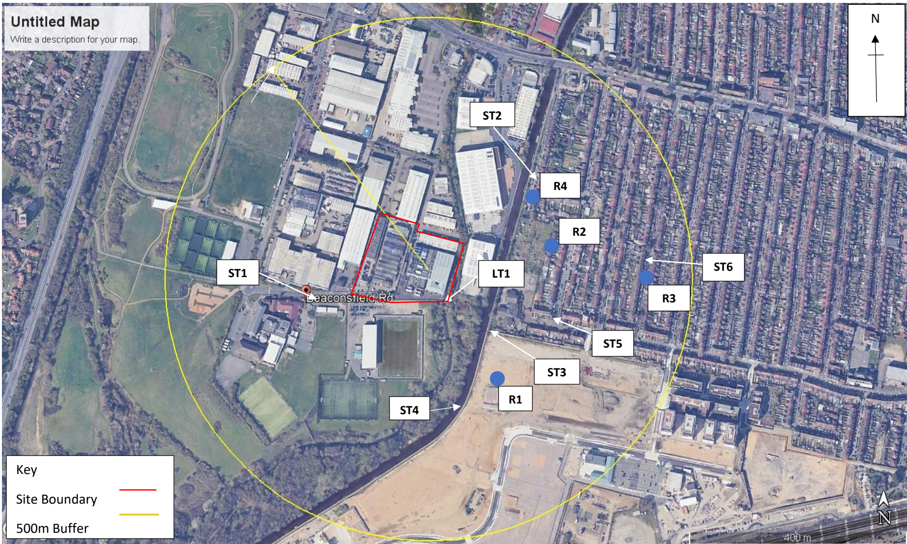
FIGURE A1: PLAN SHOWING SITE LOCATION, SOUND MONITORING LOCATIONS AND CLOSEST NOISE SENSITIVE RECEPTORS
