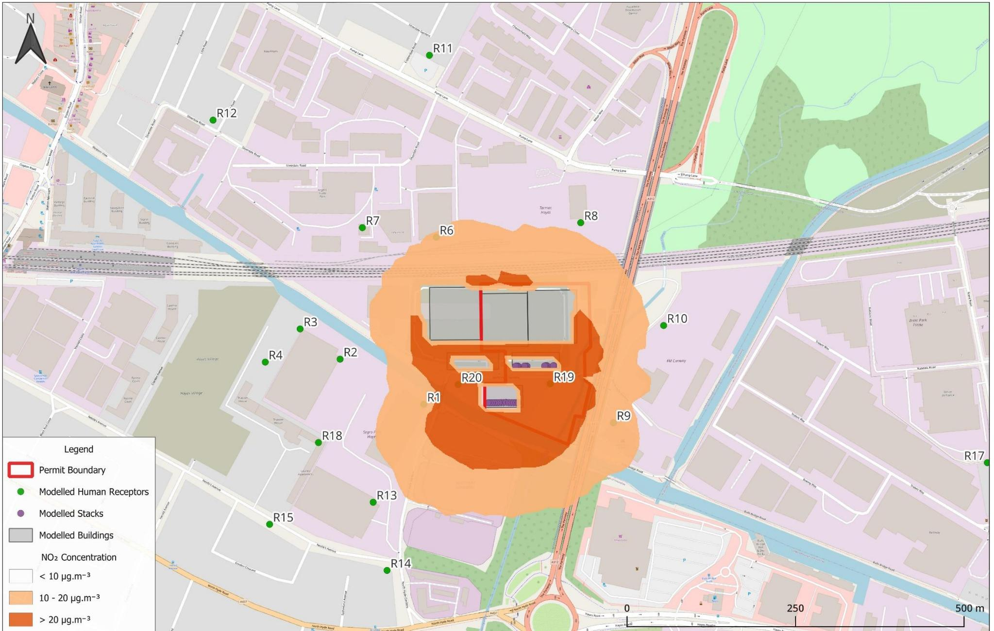
Figure 9: 99.79<sup>th</sup> %ile NO<sub>2</sub> Process Contribution - Testing Scenario 1
