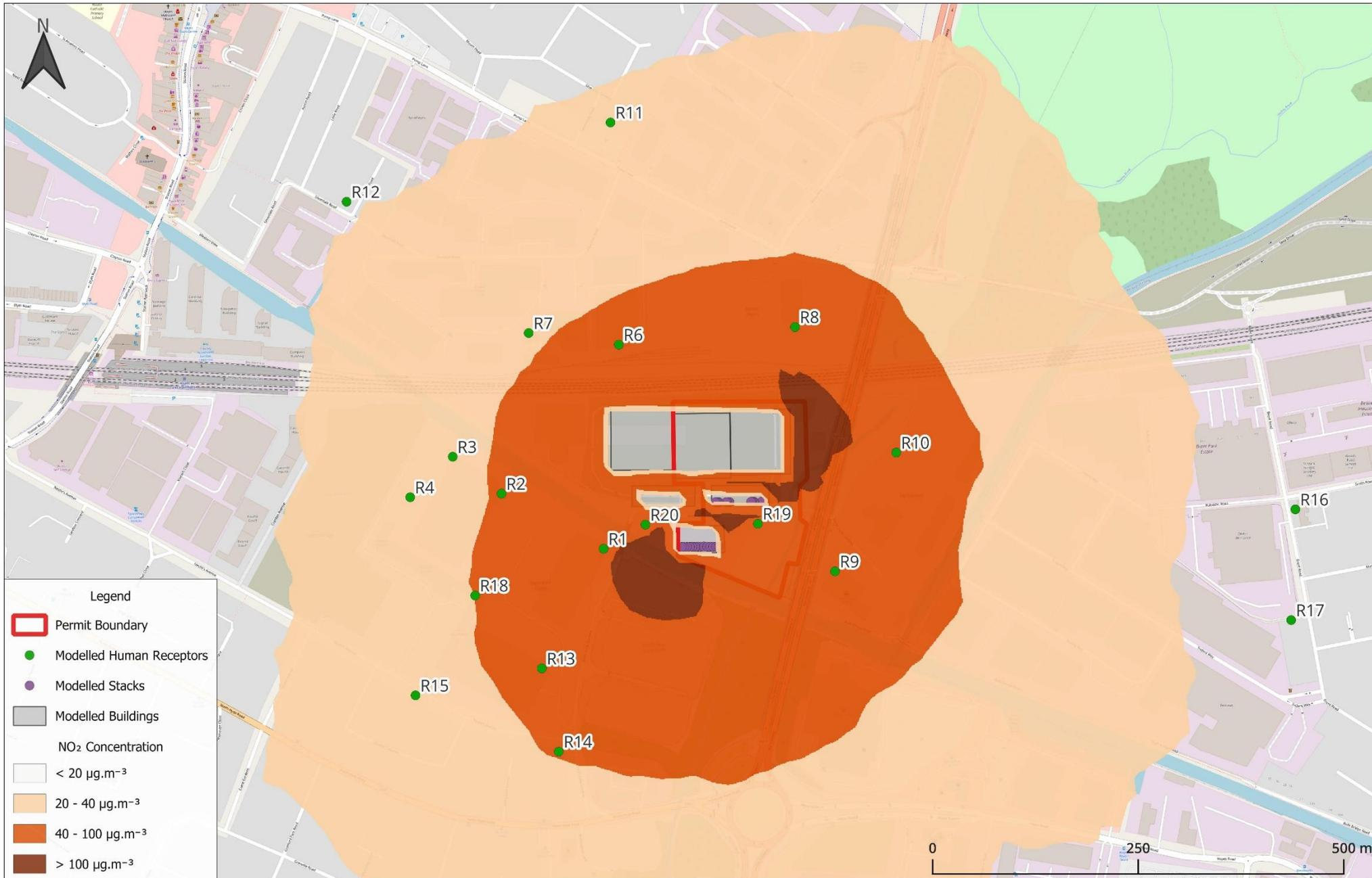
**Figure 11: 99.79<sup>th</sup> %ile NO<sub>2</sub> Process Contribution - Grid Failure**
