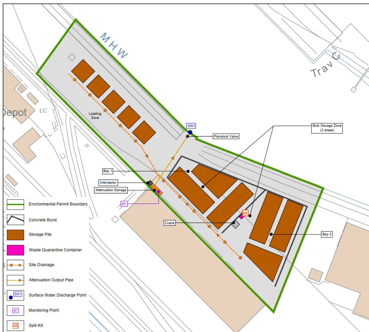
Figure 15-1 Drainage and Pollution Control
