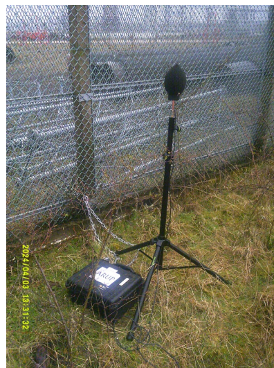
Figure 21: Measurement location U1, logger and weather station
