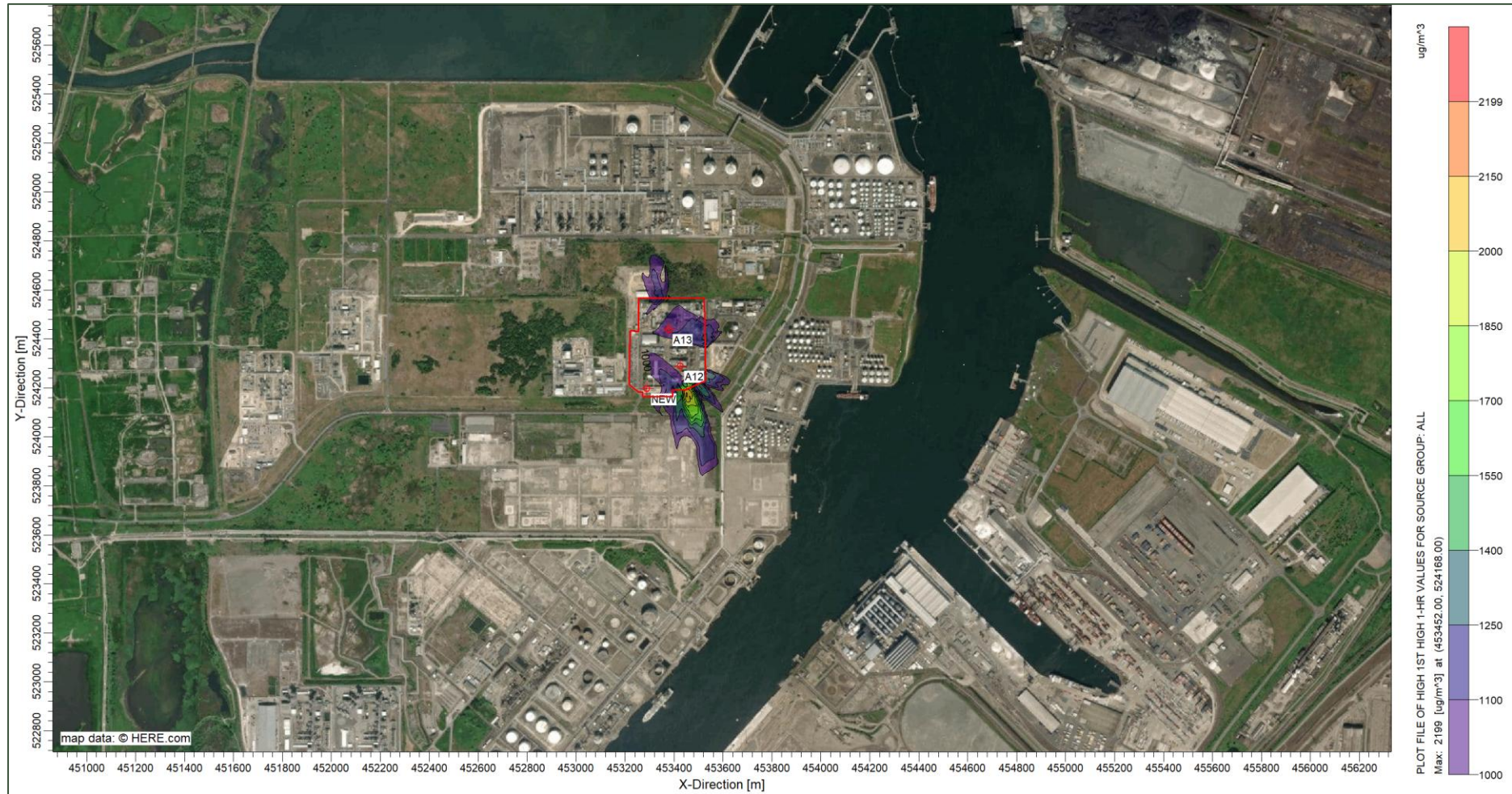
Figure A-3: MeOH Short Term (1 hour average) Process Contribution ( \mu\text{g}/\text{m}^3 )
