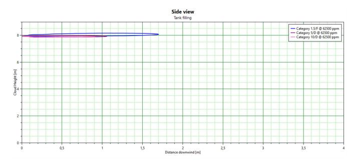
Specified mass flow rate of 1-PSV7210.4, all weather: release (incline): 45° angled from horizontal; limit for O<sub>2</sub> concentration of 19.5 Vol-% in air.
