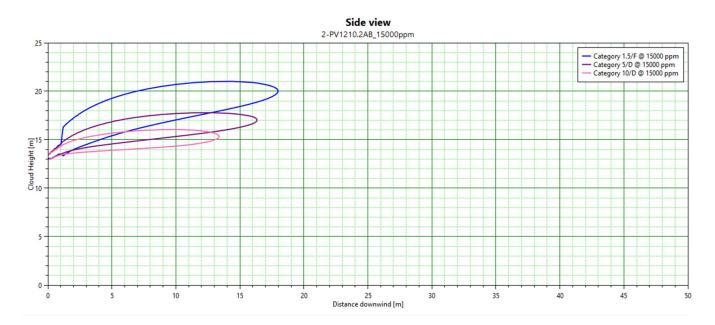
Boil off from CO2 storage tanks via 2-PV6110.1 (min. operating flow), all weather (0.5 Vol% CO<sub>2</sub> in air).
