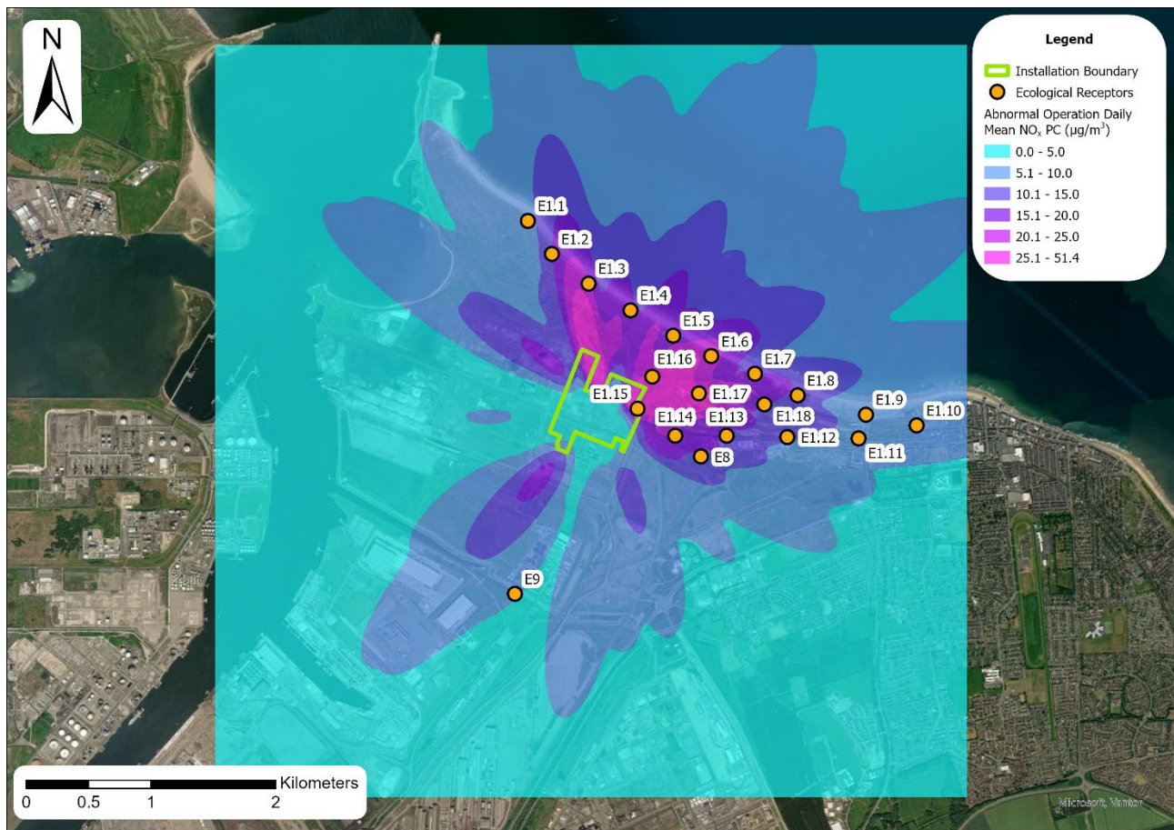
Figure 12: Scenario 2 – Abnormal Operation Isopleths of the Predicted Daily Mean NO x PCs (µg/m 3 )
