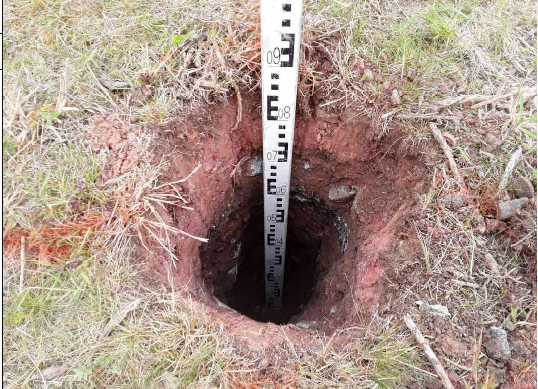
A photograph showing a borehole (BH1) in reddish-brown soil. A measuring tape is placed vertically in the hole, showing a depth of approximately 0.45 meters. The surrounding area is covered with dry grass and some green vegetation.  |
