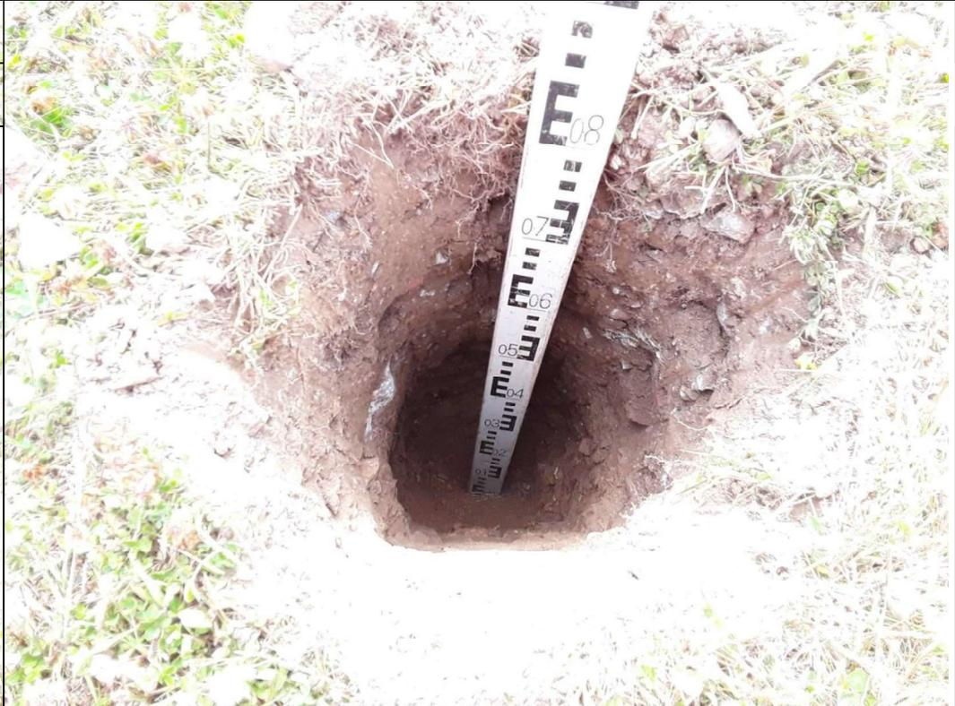
A photograph showing a borehole (BH2) in reddish-brown soil. A measuring tape is placed vertically in the hole, showing a depth of approximately 0.45 meters. The surrounding area is covered with dry grass and some green vegetation. |
