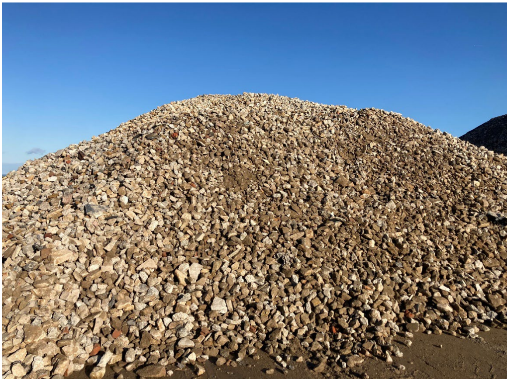
Photograph 06: Screened product following recovery. Photograph by Horizon, 11 October 2024. Note moving forwards screened product to be stored in bays.
