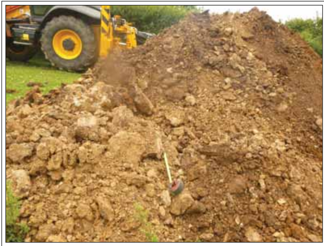
Photograph 3. Excavated spoil, Trial Pit TP02.
