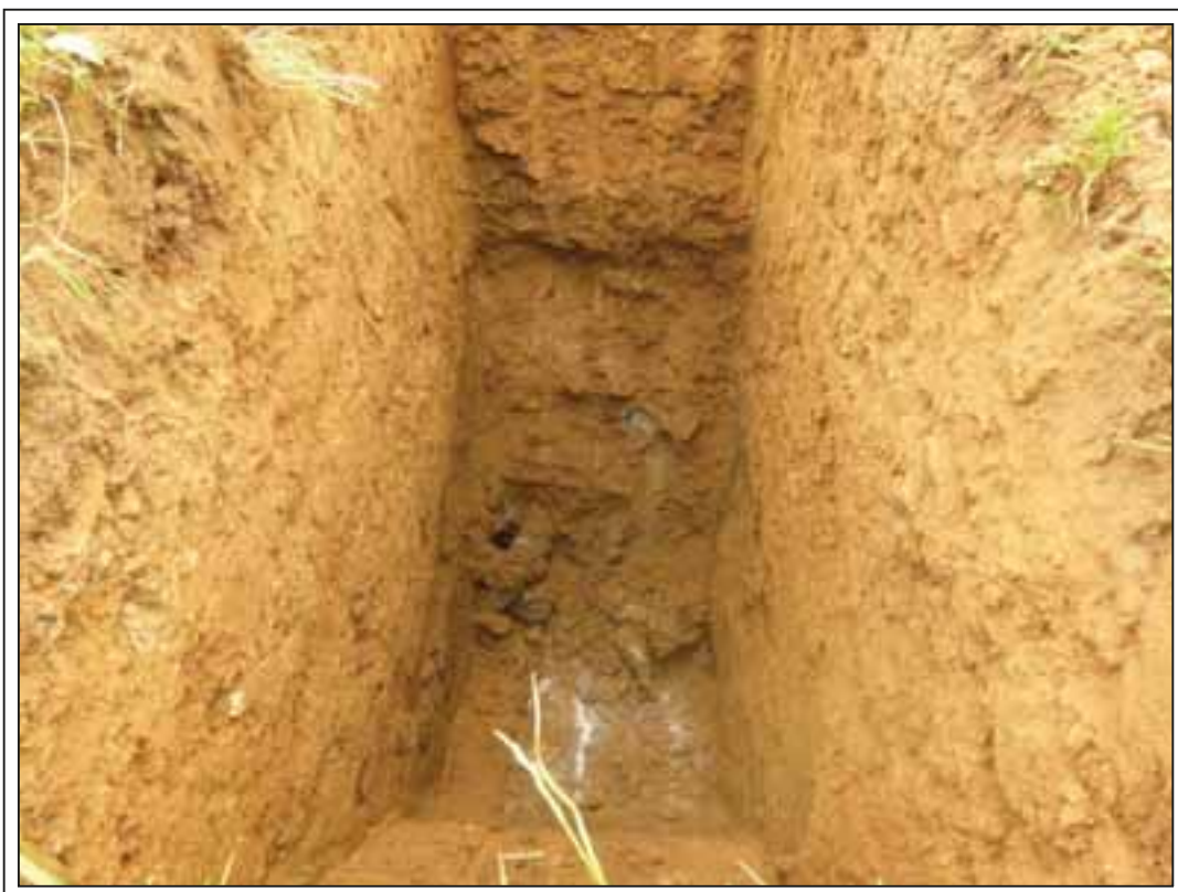
Photograph 6. Limestone cobbles and boulders (possible bedrock) exposed in base of Trial Pit TP05.
