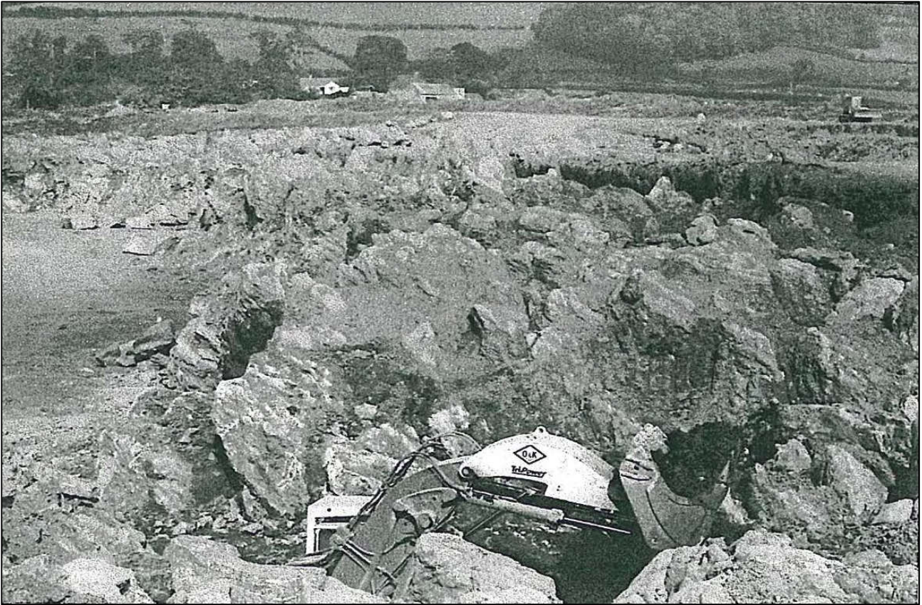
Figure 2-10 Photograph showing the northeastern area of excavation at Linhay Hill Quarry with the irregular karstic rockhead after the overburden has been stripped off. The overburden comprised superficial clays and the infill of karst features. A mechanical excavator is shown in the foreground, providing a sense of scale [2].
