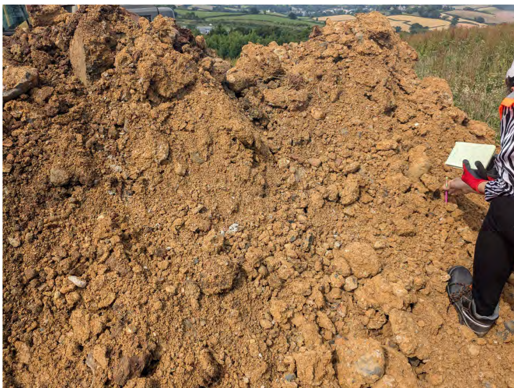
Photograph 8: View of arisings from trial pit HTP04.
