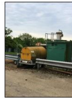
Figure 14: Portable diesel tank.
