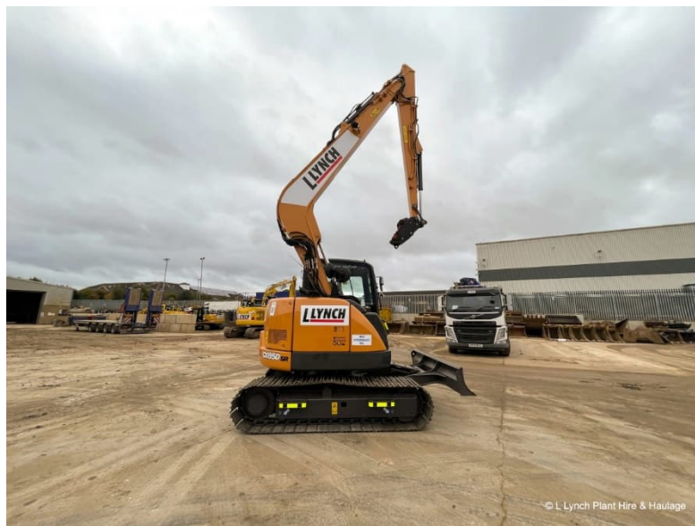
Figure 13. 9t long reach excavator
