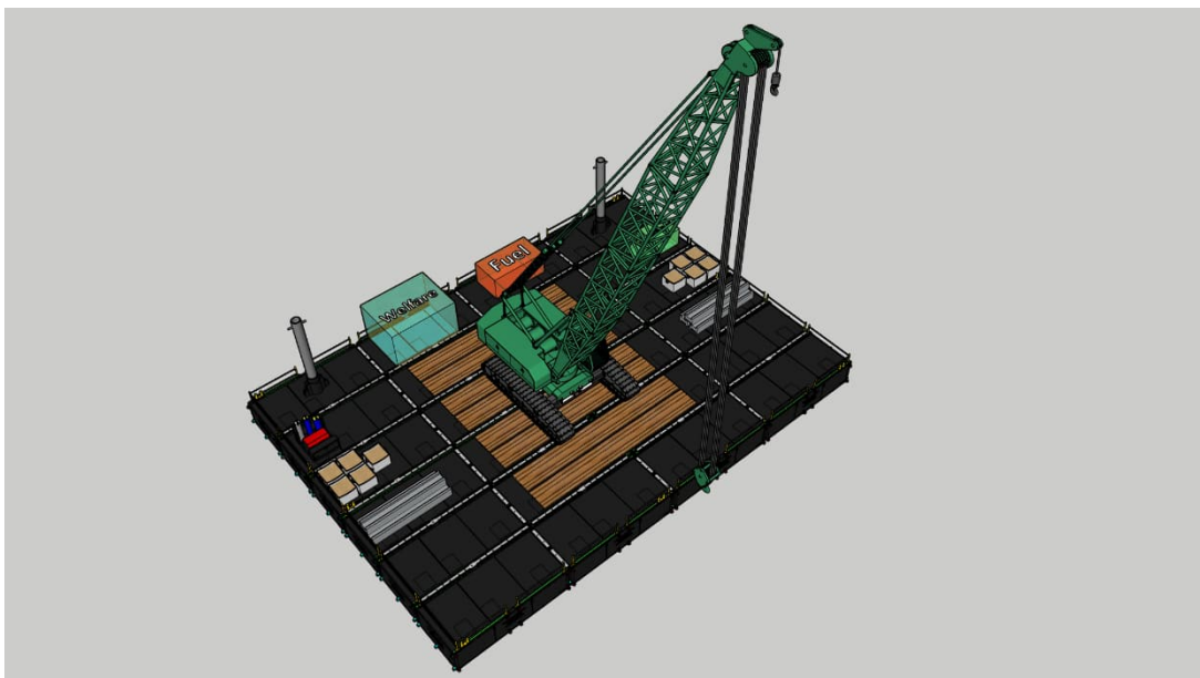
Figure 10. Mock-up of a barge with 70t crawler crane
