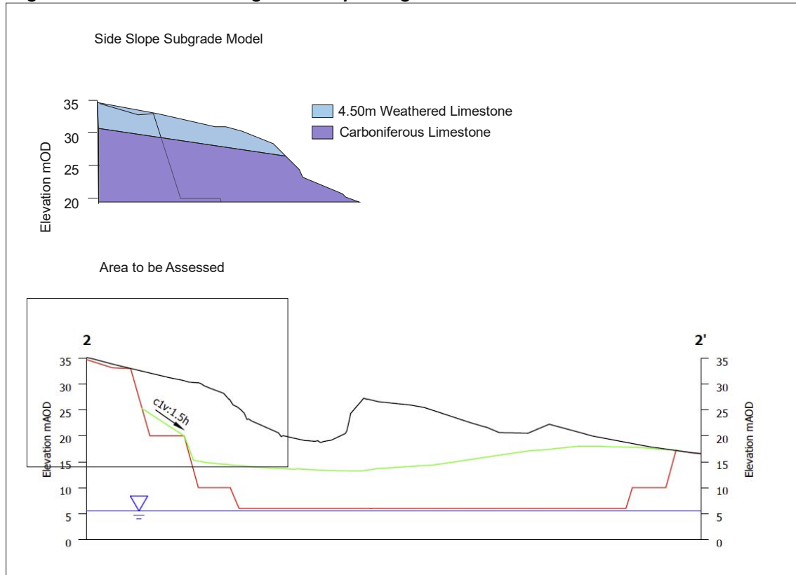
Figure SRA4 Section through side slope subgrade
